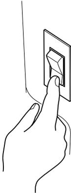
A power switch (with the breaker function) is provided on the back of the chair. A press on the right side of the switch turns on the power.
